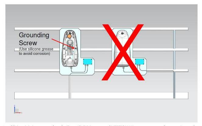
In addition, it is important that the Tron 40VDR is mounted **VERTICALLY** to ensure a good connection to the bracket module. This is important, to ensure reliable communication with the on-board VDR (Voyage Data Recorder ) computer.
