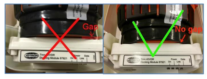
If it's a gap as shown on the left picture above, communication between VDR computer and Storage module of the beacon may be intermittent or in worst case – No communication!
