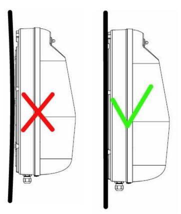
Please also ensure that the steel hull or plate where the bracket is mounted is completely flat (nor curved or uneven).
