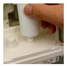
Apply the grease evenly in a thin layer as seen on the pictures on both the Docking and the Storage module (FRM- Final Recording Medium)
