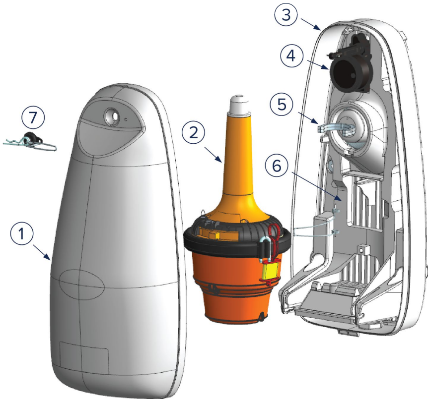
Figure 3 Illustration - Tron 40S MkII with float free bracket components
