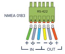
To connect to an electronic chart system, use the supplemented NMEA 0183 connector. IN and OUT in the figure is as seen from the RA10 Receiver.
