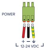
The Receiver shall be powered by a 12–24 V DC supply. Once connected, the green indicator light on the left side of the power connector will light up.
