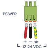
The Receiver shall be powered by a 12–24 V DC supply. Once connected, the green indicator light on the left side of the power connector will light up.
