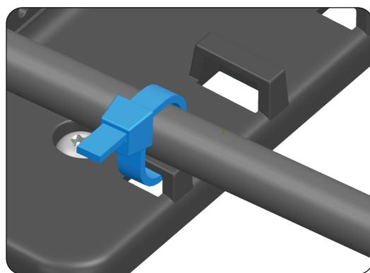
Secure the cables to the housing using cable ties.
