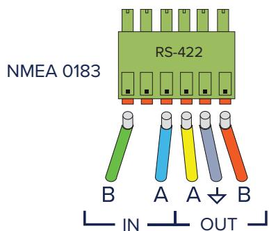
To connect to an electronic chart system, use the supplemented NMEA 0183 connector. IN and OUT in the figure is as seen from the RA10 Receiver.
