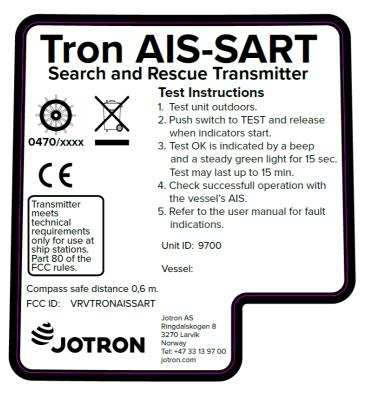
Figure 33 Image: Tron AIS-SART - Test instruction label
