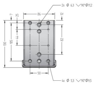
Figure 12 Illustration: Lifeboat bracket dimensions
