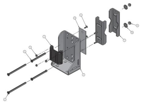
Figure 11 Illustration: Lifeboat bracket disassembled
