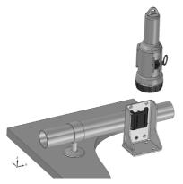
Figure 14 Illustration: Mounting on a pipe
