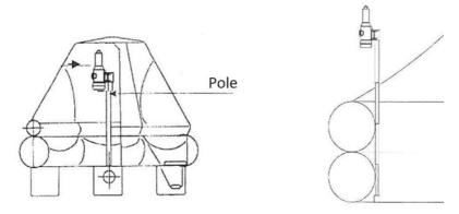
Figure 20 Illustration: using the telescopic pole on a lifeboat
