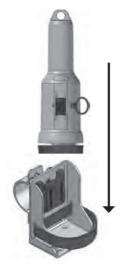
Figure 16 Illustration: Placing the Tron SART20 into the lifeboat bracket
