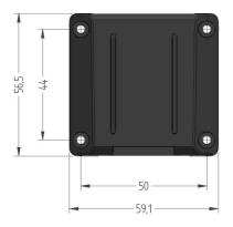
Figure 8 Illustration: Wall bracket dimensions
