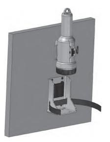
Figure 13 Illustration: Mounting - interior/exterior wall
