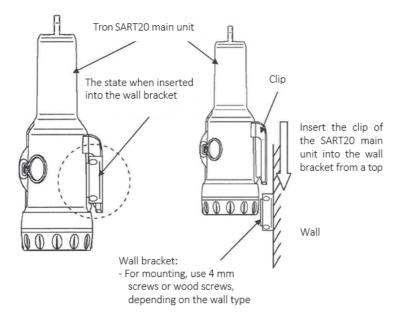
Figure 10 Illustration: Placement of Tron SART20 in a wall mount
