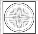
Typical display when Tron SART20 is located near (<0.2NM) the radar. Radar range is 10NM. Rings are off.
