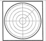
Typical display when Tron SART20 is located away (>2NM) from the radar. Radar range is 10NM. Rings are at 2NM.
