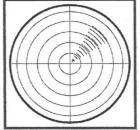
Typical display when Tron SART20 is located close (1NM) to the radar. Radar range is 10NM. Rings are at 2NM.
