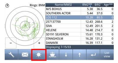
In the **Display settings** menu, you can adjust Brightness level and switch between night and day mode. Each mode has its own brightnesslevel.
