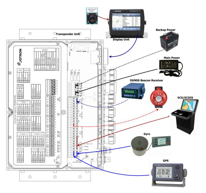
Figure 8-13: Typical Transponder connections, dashed lines shows options
