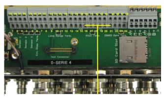
Figure 8-19 Pilot port connection, TR-8000 Transponder unit (if not used as External Display 4)
