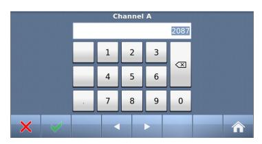
When you select either the buttons "Channel A" or "Channel B" you may input the correct channel number.
