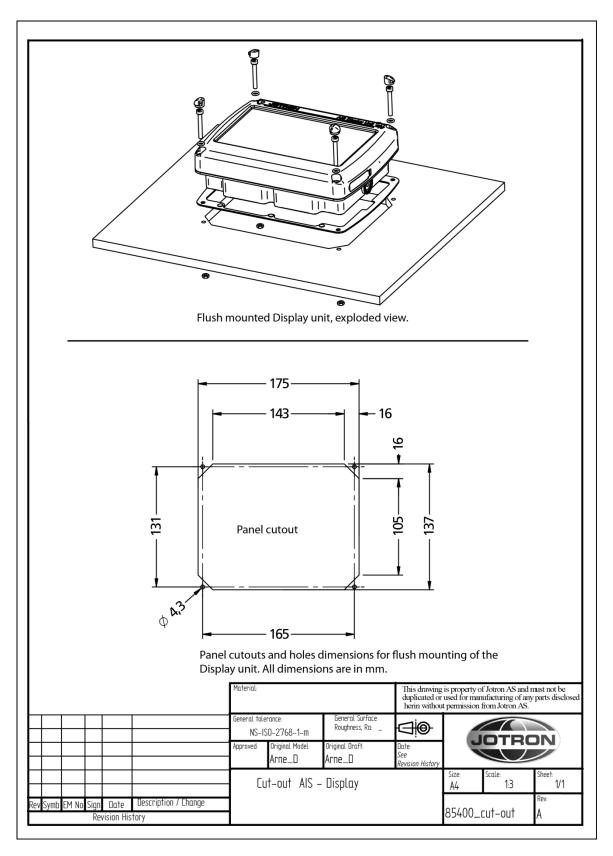
Figure 15-3 Display unit: flush mount cut-out dimensions
