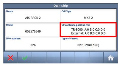
TR-8000 -> means position of the antenna connected directly to the transponder.
