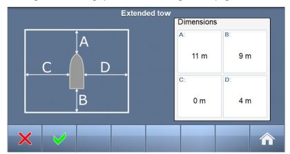
The extended dimensions are added to your vessel existing physical dimensions creating a larger virtual vessel. Other vessels will see your vessel as larger, as this virtual size is broadcast in message 5.
