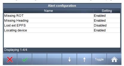
During installation it is possible to disable some specific alarms. Disabling alarms is done by selecting one alarm and clicking the Toggle button.
