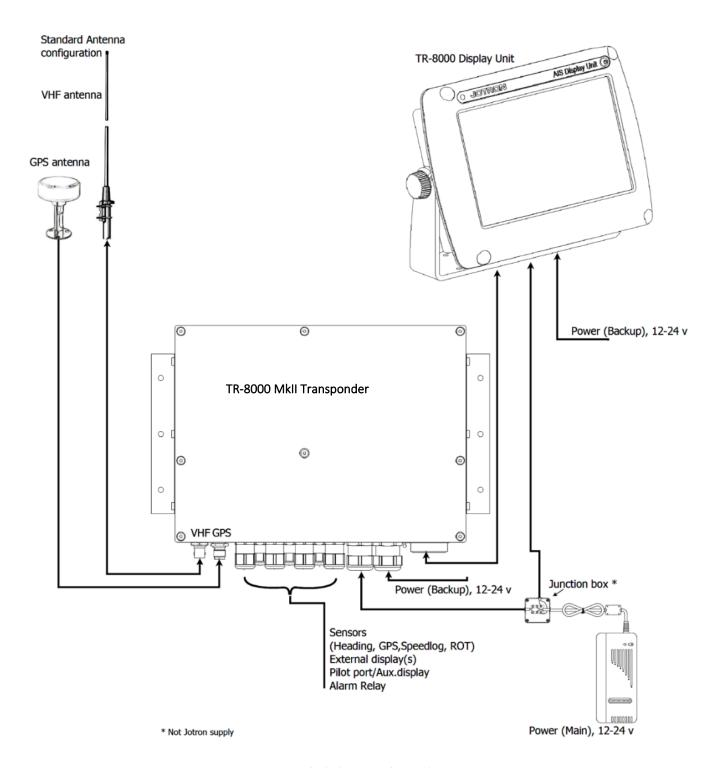
Figure 8-10 Block diagram of typical connections
