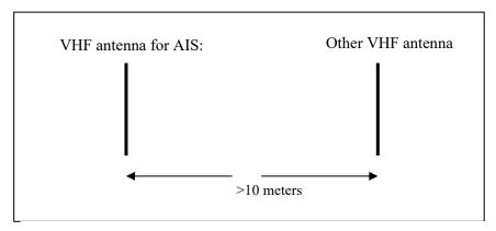
Figure 8-5 Horizontal separation distance.
