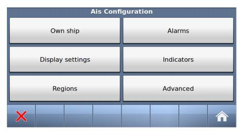
The AIS configuration menu consists of six menus, containing the settings and configurations most applicable to the user. Some settings are write-protected by administrator password, but the user is always allowed to view the current settings.
