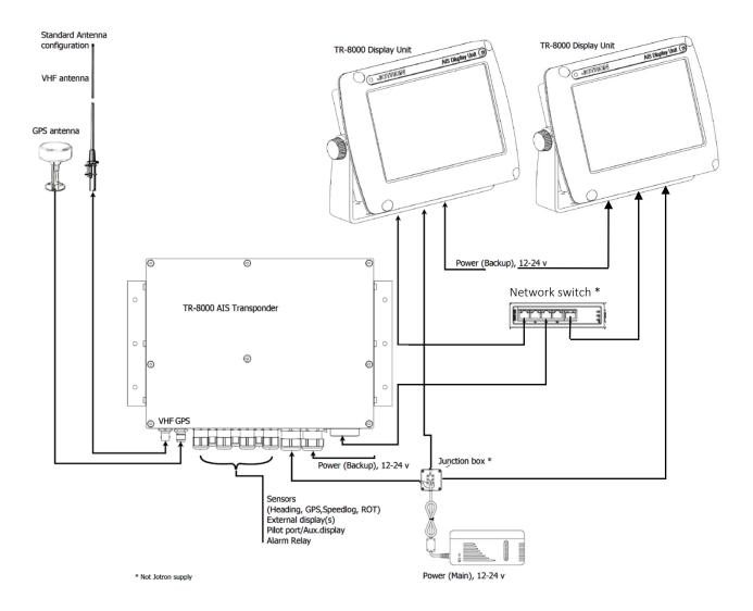
Figure 8-11 Block diagram of Dual Display connection
