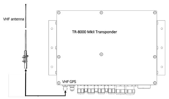
Figure 8-8 Connection of VHF antenna
