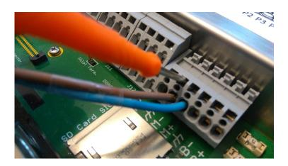
Figure 8-8-16 Use the supplied orange screwdriver to open the terminals.
