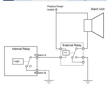
Figure 8-24 Typical Alarm connection
