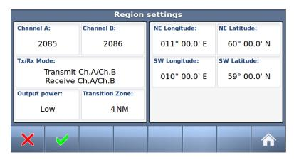
For Custom defined Regions (Either configured by the operator or configuration is received from an AIS Base Station in a special message) the Region have in addition North East position and a South West position defining the area in which the special settings of:
