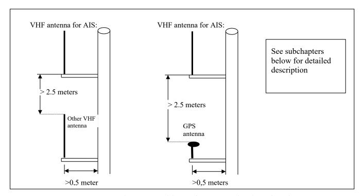
Figure 8-6 Vertical separation and distance from mast or other object of metal
