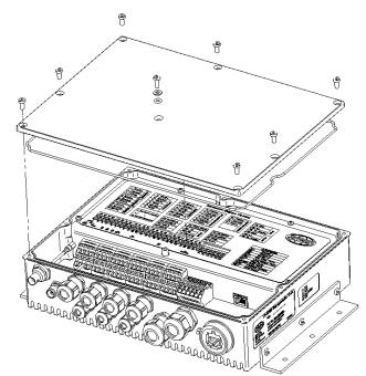
Figure 8-1 Transponder unit: exploded view
