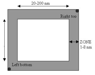
This zone is used for frequency transition so only one frequency is changed at a time. There are defined rules for how the AIS will behave through this zone.
