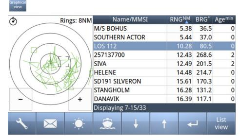
anchored/moored, the North Up configuration will automatically be chosen. If a valid heading is received from external heading sensor (Gyro, Satellite compass or similar), own ship will be oriented according to this. If heading is lost, Course Over Ground (COG) will be second choice for own ships orientation on the display.
