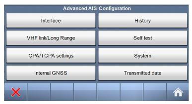
The **Advanced Menu** is intended for use during setup and maintenance of the AIS system. Some of the menus are write protected by password, but all parameters are readable to all users for inspection.
