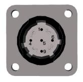
Figure 8-28 AMP 206486-1 Pinout
