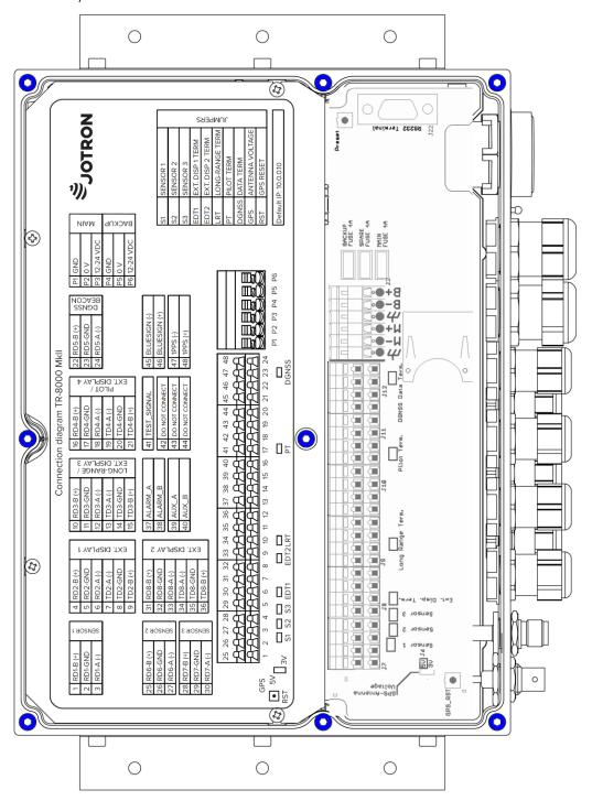
Figure 8-12 Transponder with lid removed, lid screws highlighted
