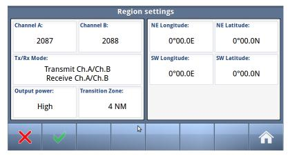
When "Add Region" is selected, default values for Channels, Tx/Rx Mode, Power and Transition zone are configured, but all these parameters may be altered together with defining position of the North East and South West corners of the Region.
