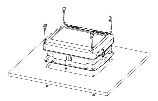
Figure 8-4 Flush mounted Display Unit, exploded view.
