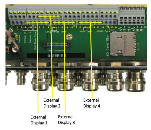
See also chapter 10.6.1.2 which describes how to configure "External Display" options and table in chapter 8.3.2.2 for details of pinouts.
