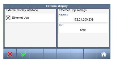
If Ethernet is used, an external Ethernet switch is required for simultaneously connection of the display unit and a remote computer, see also chapter **8.3.2.5** which describes the External Display physical connections.
