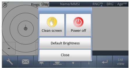
When the ON/OFF button is pushed and released, a popup menu is displayed with some display options. Additionally, if the brightness is low, it will automatically be increased. This feature can be used if the user by some reason has too low visibility to adjust the brightness the regular way. If the Default Brightness button is pressed, the brightness will be set to a 50% value. Otherwise the current brightness level will be restored when the dialog is closed.
