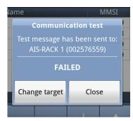
If the TEST fails, we can select another target and redo the test
