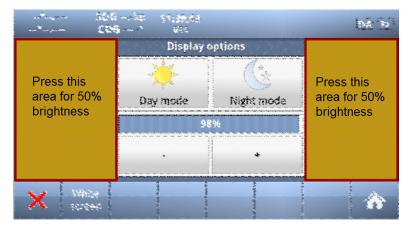
Touching the empty area at the left or right side of the display restores a 50% brightness level if the display gets too dark to see the actual buttons for this purpose.
