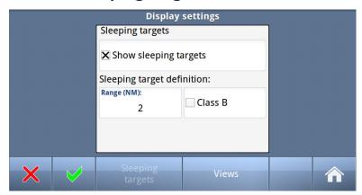
The first "Display settings" menu configures "Sleeping targets". Sleeping target has a smaller shape and no vector in order to display a less cluttered graphic view. Sleeping targets can be defined to be all vessels outside a defined range, and/or all class B stations.
