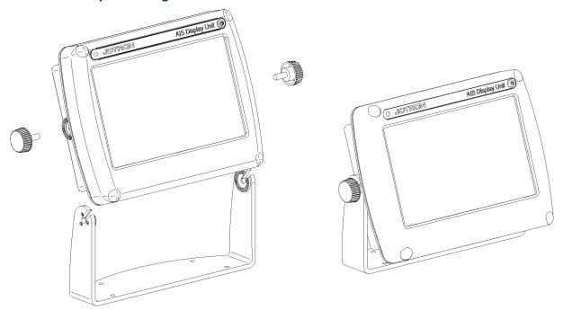
Figure 8-2 Desktop mounted Display Unit
