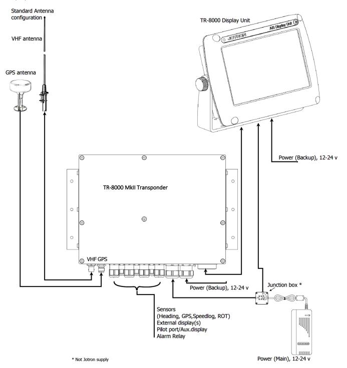
Figure 6-1 Block diagram of TR-8000 MkII system
