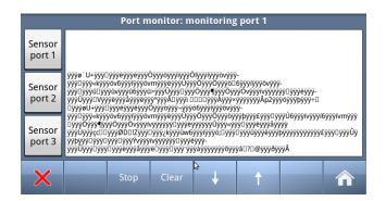
The two screenshots above shows Sensor data which are most probably OK, while left screenshot shows corrupt data from incorrectly connected sensor (Polarity of signals are incorrect)
