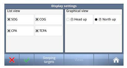
Press the View button on the button bar in order to configure how the ship list and the graphic view should be displayed.
