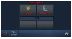
In the low brightness end of the scale, the steps are more accurate to adapt to very low intensity levels.
