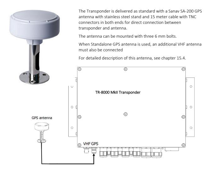
Figure 8-7 GPS antenna connection
