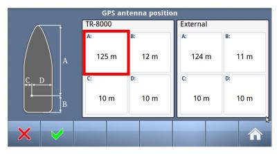
Click on "A"-"D" for "TR-8000" and "External" and input correct values. The length and width of the ship will automatically be derived from these values.
