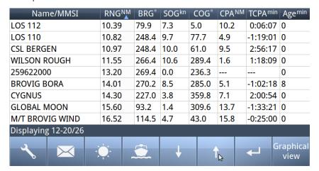
Note that in areas with heavy traffic, the number of received Vessels can be large. In cases where more than 200 vessels are received, the display unit will at any time display the 200 nearest vessels. Display of other types of objects (base stations atons etc.) will not be restricted in any way. This restriction also affects the graphical view described in the next section. The output to external devices (ECDIS,Pilot) is not affected by this filtering.
