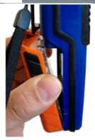
3. Squeeze in the black battery clips on either side of the battery to lock the battery into place.
