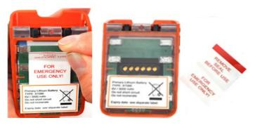
2. Using the fixing track, attach the emergency battery onto the back of the Tron TR30 AIR radio.
